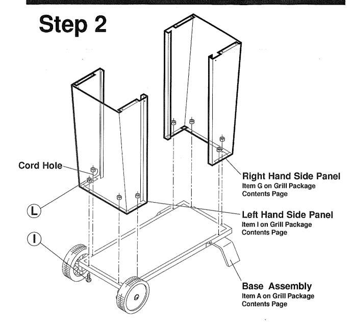
Left and Right Side Panel Assembly Install the left hand side panel and right hand side panel onto the base assembly using 4 of item I and 4 of item L. Tighten all fasteners using a L-hex Wrench and a 10mm box type wrench.
